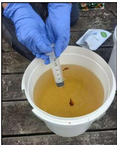
Water samples were collected from the fish passage (above left) which runs under the predator-proof fence, allowing fish to move freely between two parts of the wetland. Samples were also taken from various other areas. Via a syringe (left) they were put into sealed vessels and into a bag, on which was recorded details of the collection point (right).
